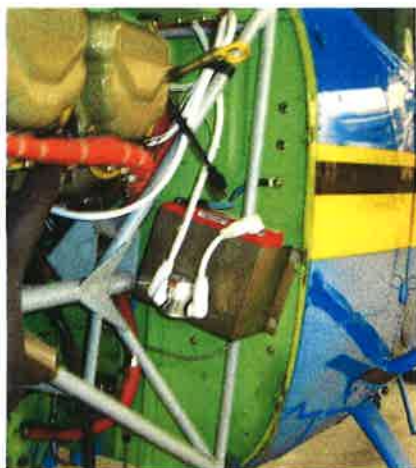
PHOTO 3.2: Canted Inst'll with Seaplane Typical Engine Mount.
