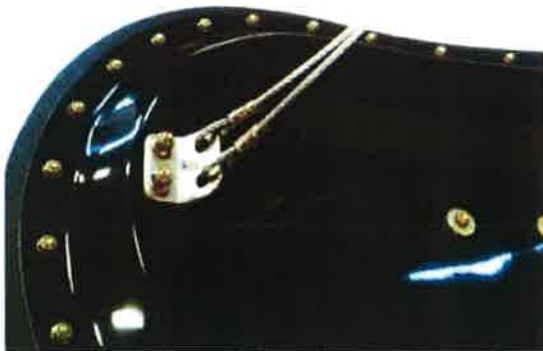
Front Cable Assembly to Front End of Ski
