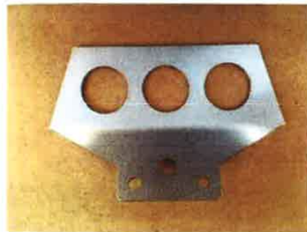
Figure 2 FAD P/N 3232W-2 Rear Seat Weld-On Shoulder Harness Attach Bracket
