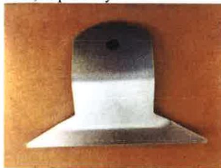
Figure 1 FAD P/N 3232W-1 Front Seat Weld-On Shoulder Harness Attach Bracket
