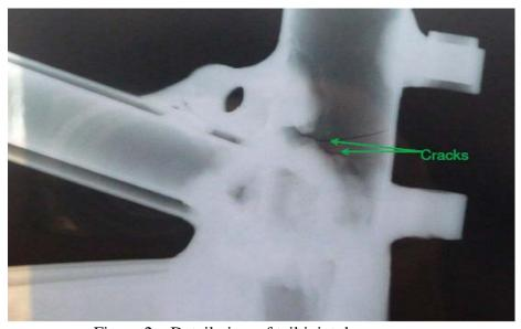
Figure 2 – Detail view of tail joint damage area
